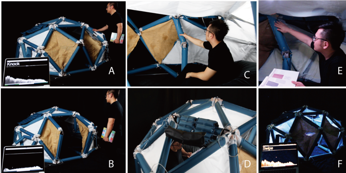
Fig. 4. (a) shows a user performing a knock gesture and our system recognizing user input; (b) shows the door opening for the user to enter.(c) shows a user performing a squeeze gesture; (d) shows the windows of the dome rolling up in response.(e) shows a user performing a swipe gesture; (f) shows the lighting switched on inside the dome.
