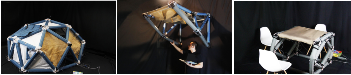
Fig. 1. (a) A geodesic dome that deploys itself upon inflation and has embedded actuation and acoustic sensing to open its doors and raise its windows; (b) a canopy with a controllable venetian blind via capacitive sensing; (c) a portable table inflated on-demand via a pressure sensitive control. All of our structures have embedded actuation and sensing that support a range of interactions (e.g., a user performs a knock gesture on the dome’s door and the door swings open).
