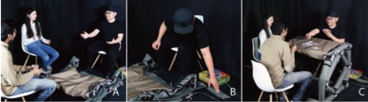
Fig. 9. A deployable table with a user triggering the structural members' inflation with an embedded pressure sensor.
